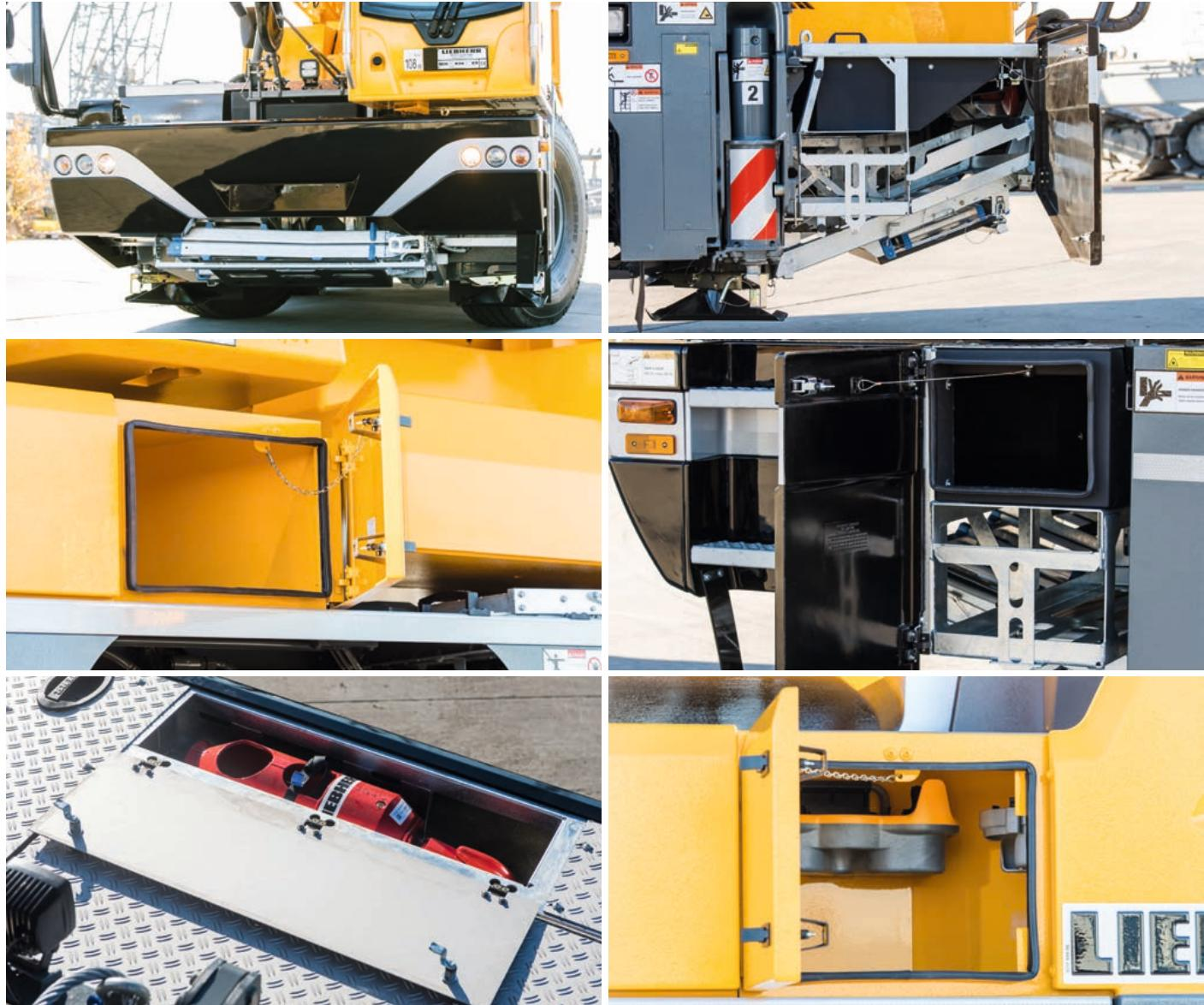
The LTC 1050-3.1 carries all the equipment it needs on the crane. With an axle load of 26,455 lbs it can drive with the basic ballast of 14,330 lbs and the folding jib. The spacious storage compartments provide space for additional equipment.
