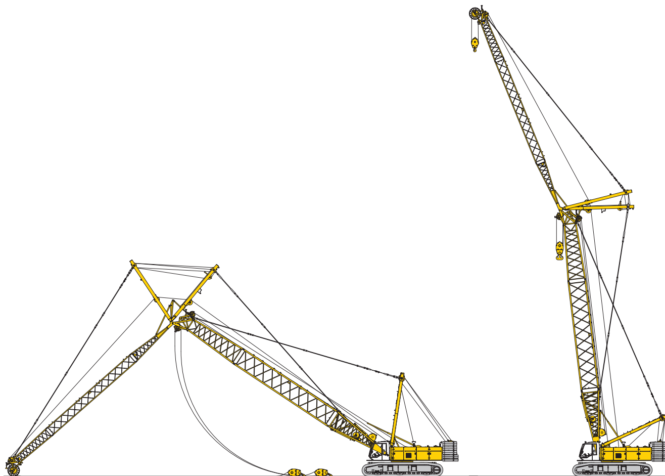
Erecting of main boom and luffing jib
